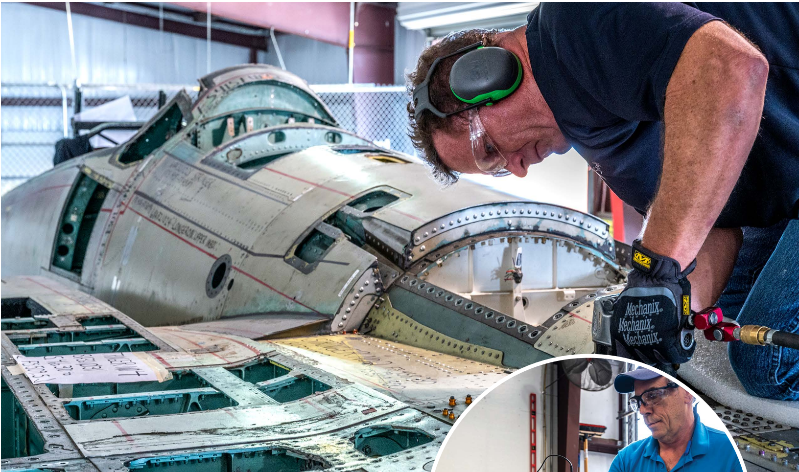
F-15 teardown and corrosion research.
